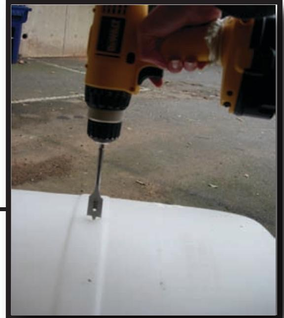
**Step 3:** Using the 9/16" drill bit, drill an opening for the stopper at the very bottom edge of the barrel.
