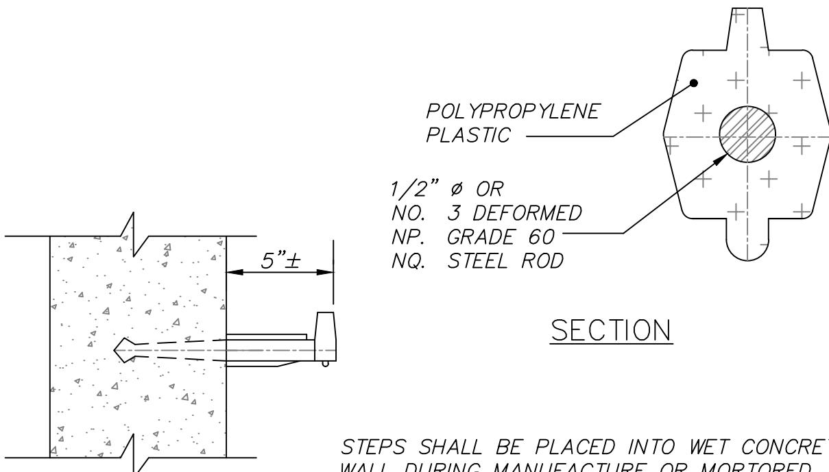
STEPS SHALL BE PLACED INTO WET CONCRETE
