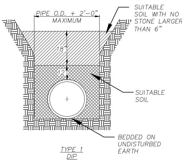
COMPACTED BACKFILL 95% OF THEORETICAL MAXIMUM DRY DENSITY WHEN UNDER PAVEMENT
