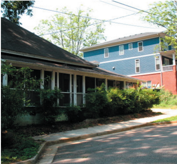
Figure 44 - The scale contrast of the three-story infill dwelling uphill to its one-story historic neighbor is exacerbated by the unbroken side plane of its rectangular mass.
